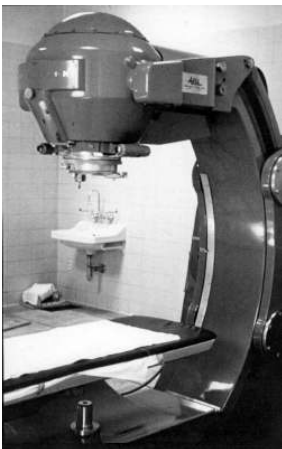
First supervoltage radiotherapy unit in NZ: AECL Theratron-B Co-60 isocentric unit, 75 cm SAD; installed at Christchurch Hospital in 1956
