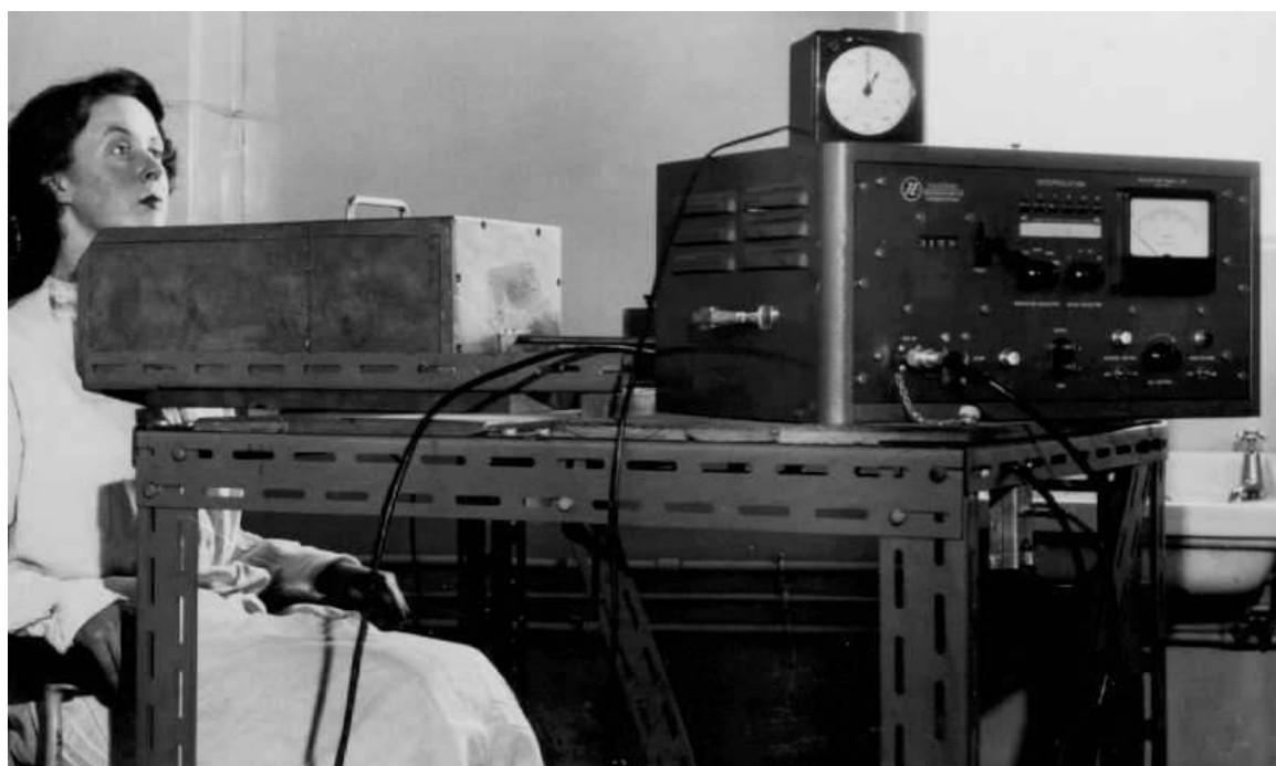
I-131 thyroid uptake equipment, 1952, as developed by Thyroid Research Unit, Otago Medical School. Two G26.Pb geiger tubes; 25 mm lead-walled 'castle'; perspex neckbar; good geometry, with 20 inches (50 cm) distance from geiger tube to neckbar; Note binary '64 Scaler' with separate timer. 'Patient' seated in dental chair
